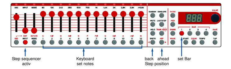
Sequences of the OSCILLATOR track can either be recorded in real time via MIDI or the note keys or programmed in EDIT mode while the sequencer is running. The step sequencer is 4-beat and has up to 32 steps per measure. You set this grid with the RESOLUTION control of the SHOT section.
