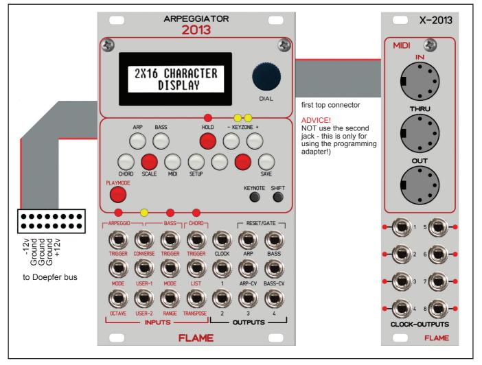
The module is delivered with a connected ribbon cable for the Doepfer bus. The red lead marks -12 volt. Connecting the module please note the right polarity!
